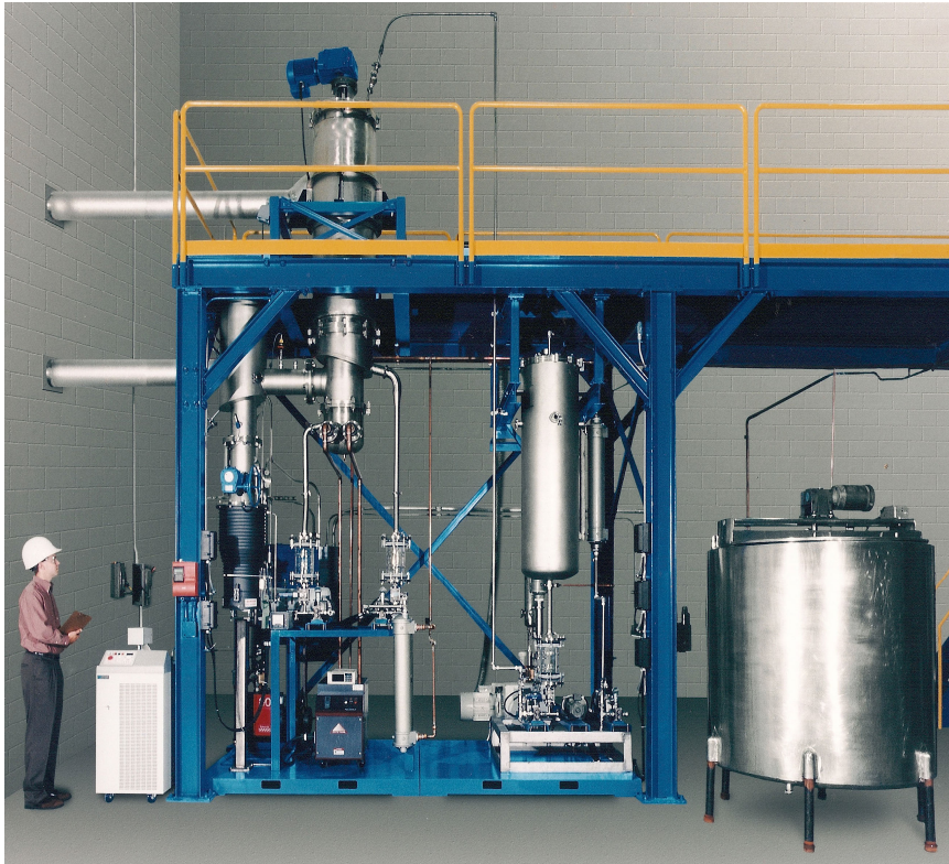
Pope Scientifics' 20" Wiped Film Molecular Still with Passive Degasser Toll Processing Unit.
