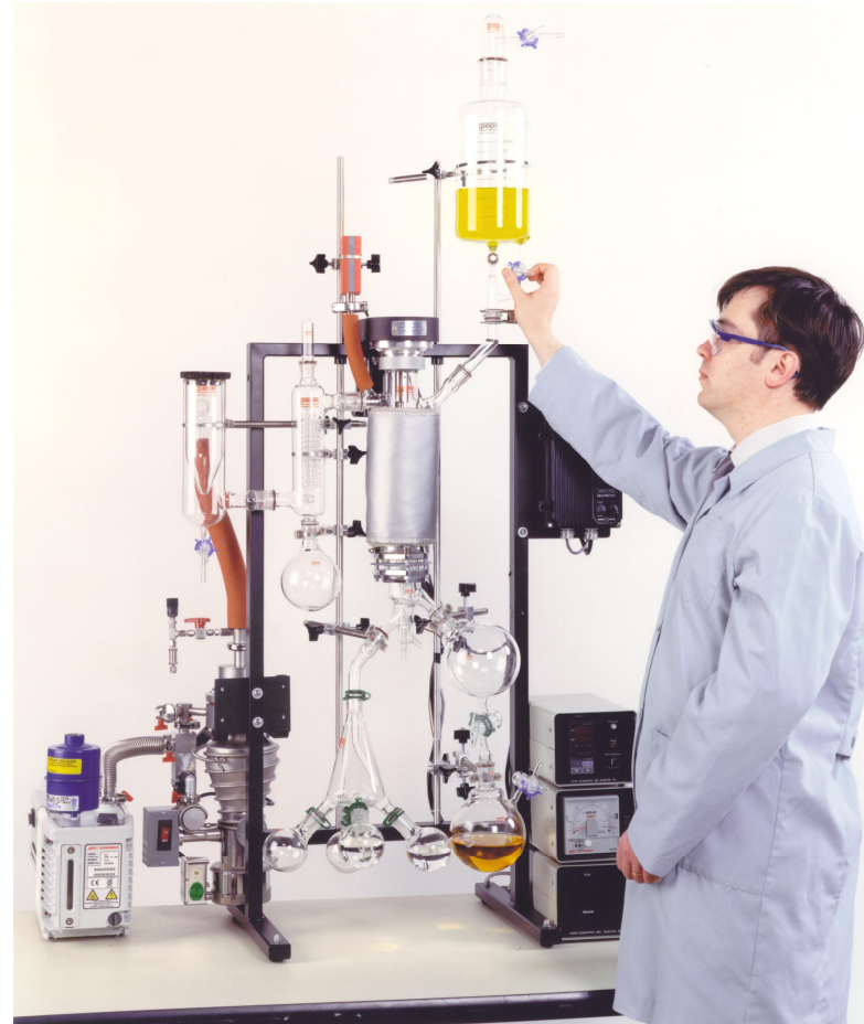
2" Bench Top Glass Wiped Film Molecular Still with optional Additional External Condenser
