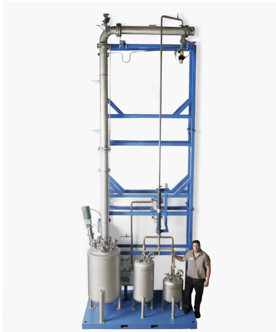
6" Diameter Column Batch Distillation Pilot Plant
