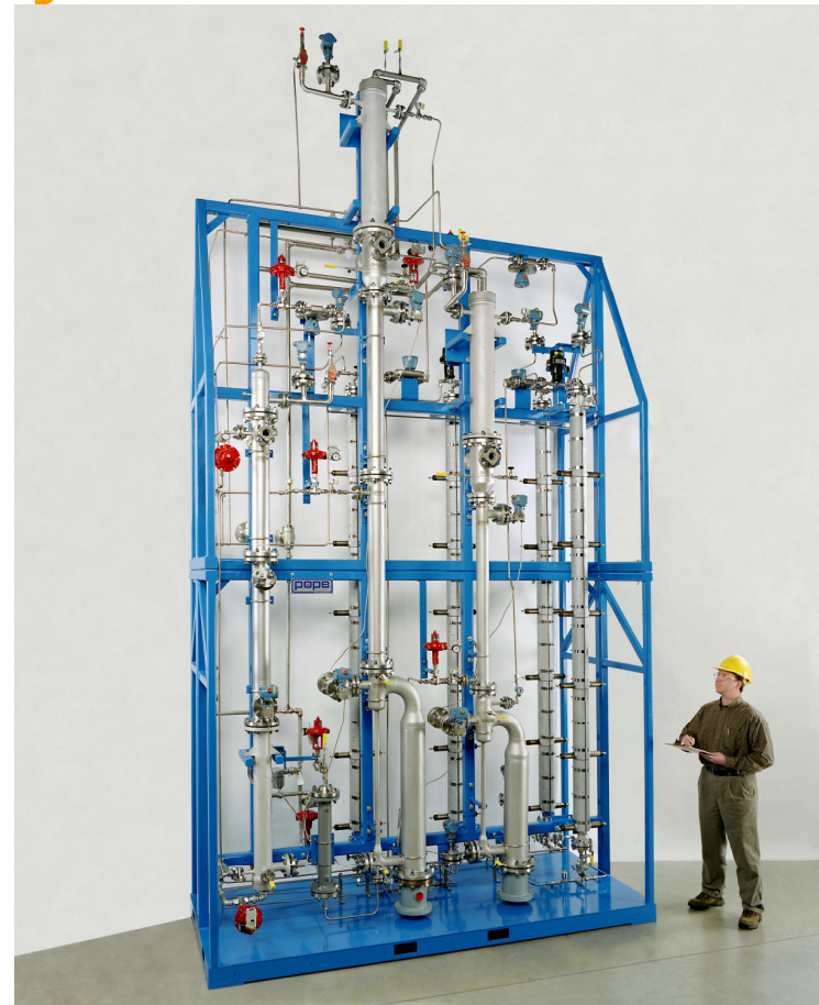
2 Stage Continuous Distillation Pilot Plant
