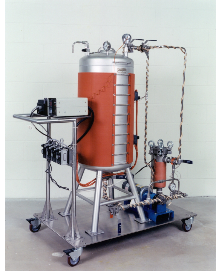
Heated Reactor / Filter System
