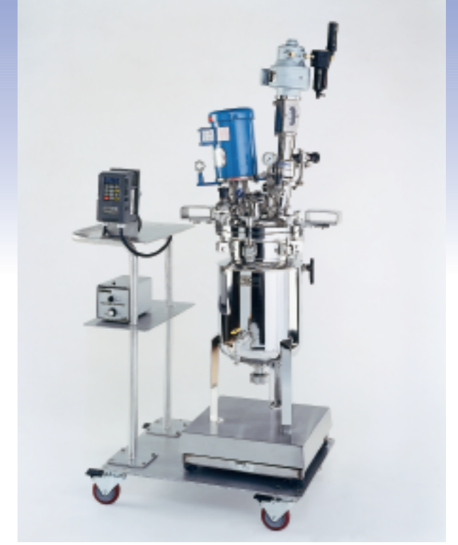
5 Gallon Homogenizer/Blender System for pharmaceuticals, includes instrumentation, scale, and heater/chiller system (not shown).
