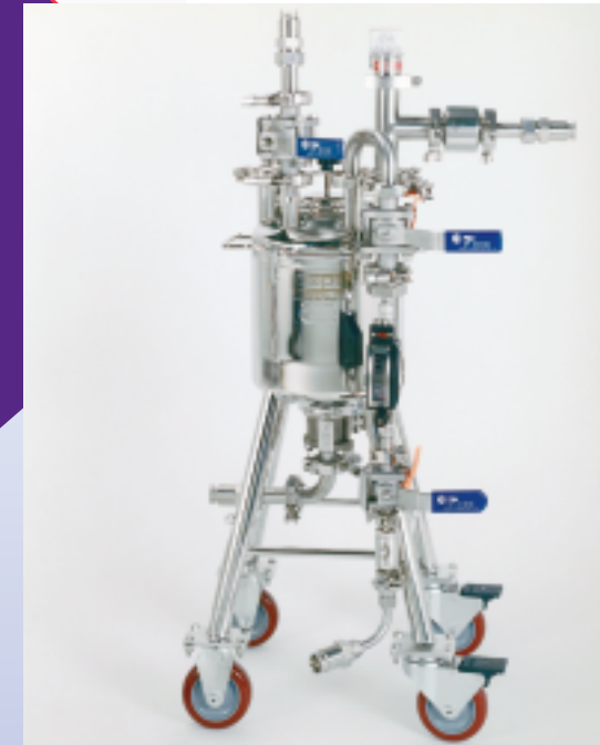
10 Liter Portable Pharmaceutical Process/Transfer Vessel with sparging control, check valves, quick connections, rupture disk.
