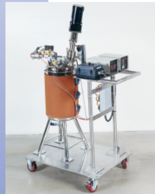
10 Gallon Hydrogenation System for high purity speciality chemical processing.
