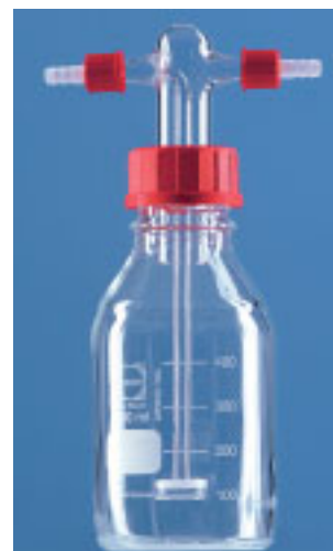
Gas Washbottle to Drechsel with Filter Disc
