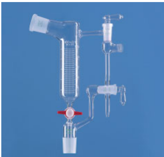
Distilling Receiver to Anschütz-Thiele, Bent, PTFE Stopcock
