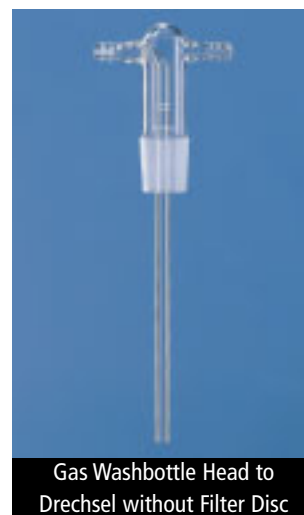
Gas Washbottle to Drechsel without Filter Disc
