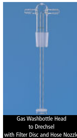
Gas Washbottle to Drechsel with Filter Disc and Hose Nozzle
