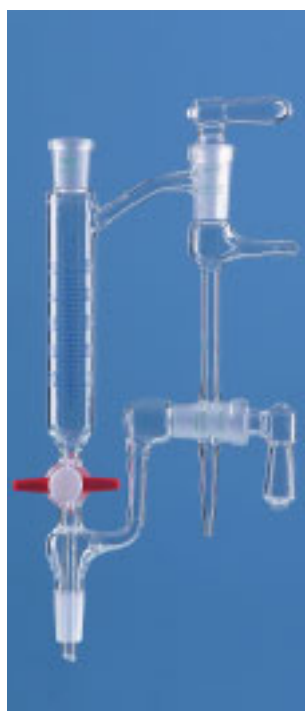
Distilling Receiver to Anschütz-Thiele, Straight
