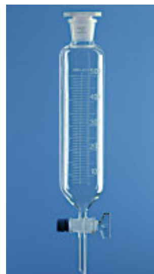
Separating Funnel, Cylindrical, with Glass Plug
