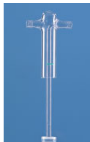
Gas Washbottle Head to Drechsel with Filter Disc
