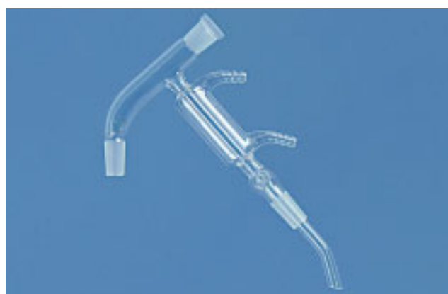
Distilling Link for Short Path Distillation
