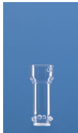
Extractor Distribution Tube for Specific Heavier Solvents
