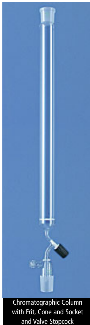
Chromatographic Column with Frit, Cone and Socket and PTFE Stopcock
