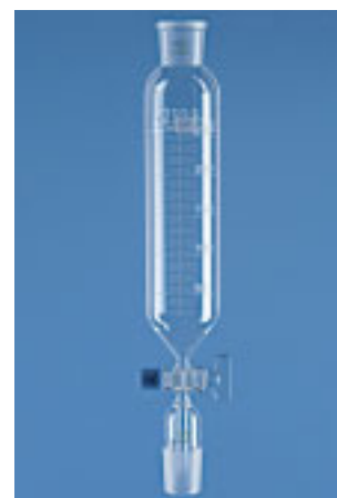
Dropping Funnel, Cylindrical, with Glass Plug
