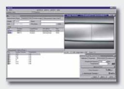
The DSA2 controls the rotational speed of the capillary and determines the diameter of the rotating droplet in realtime.
