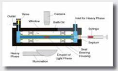
A droplet located along the axis of a rotating capillary filled with denser fluid will form a cylindrical shape. With the appropriate drop volume and rotational speed, the drop
