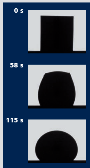
Image recording of the smelting process with accompanying contact angle measurement
