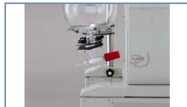
The drain valve realizes easy continuous operation.
