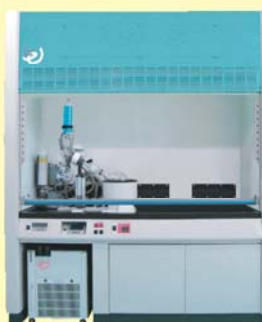
Built-in condensing system in fume hood (Custom design example)
