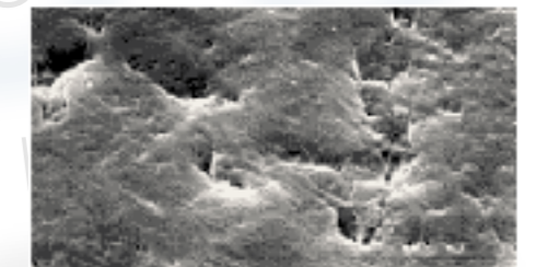
PTFE surface: before plasma treatment
