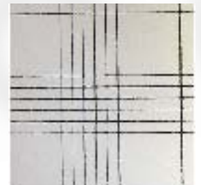
Grid cut test on PBT: with plasma treatment
