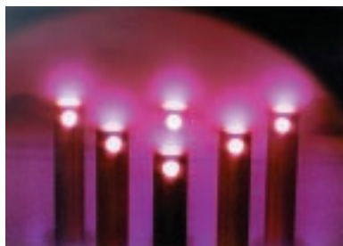
Plasma cleaning of copper tubes
