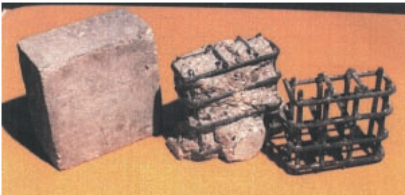
Above: Aggregate that has been freed of cement by powerful acoustic waves; left: extracted reinforcements
