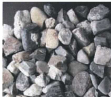
Above: Aggregate that has been freed of cement by powerful acoustic waves; left: extracted reinforcements
