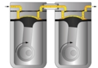
1. Condensation reduces pump efficiency
