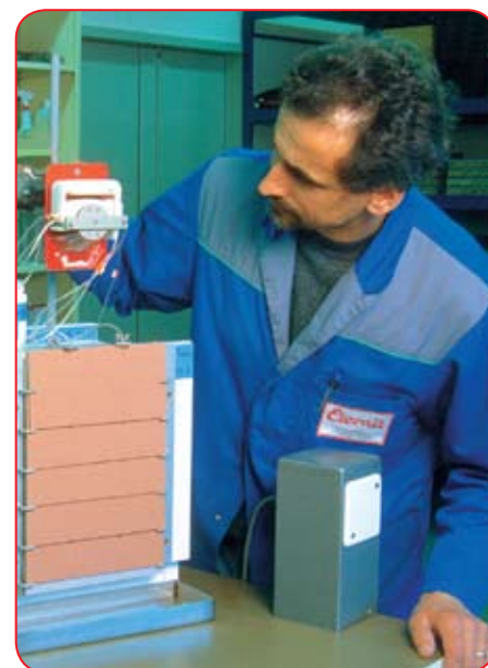
Long-term determination of environmental influences on asbestos-cement
