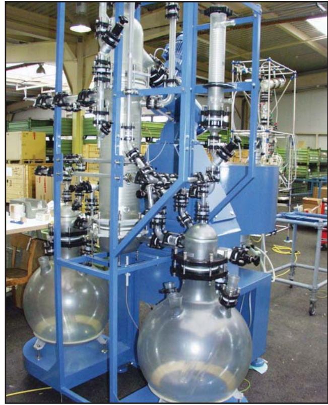
Fig. above: glass parts with dissipative coating.
