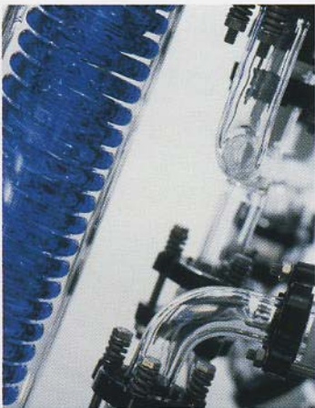
▲ QVF coil-type heat exchanger for high purity
