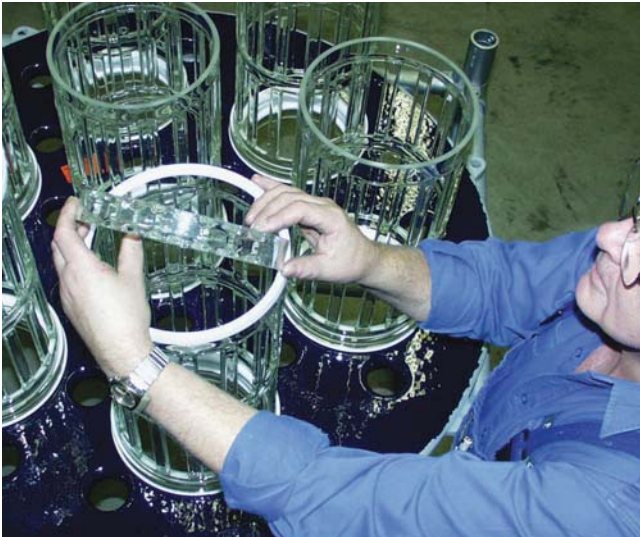
Fig.: CORE-TRAY DIN 1000 assembly, here for packing with glass support
