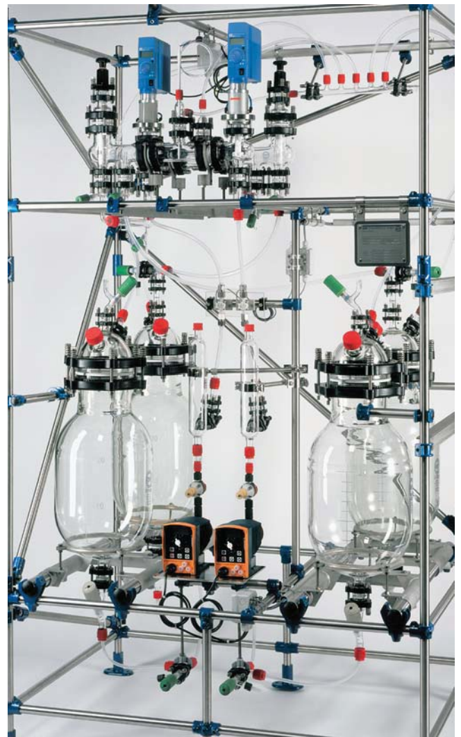
Fig.2: Two-phase mixer settler apparatus DN 50
