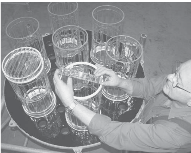
Fig. 1: CORE-TRAY DIN 1000 assembly, here for packing with glass support
