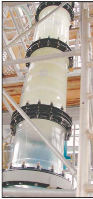
Fig.: Plate structure, segmented packing, installation in glass columns
