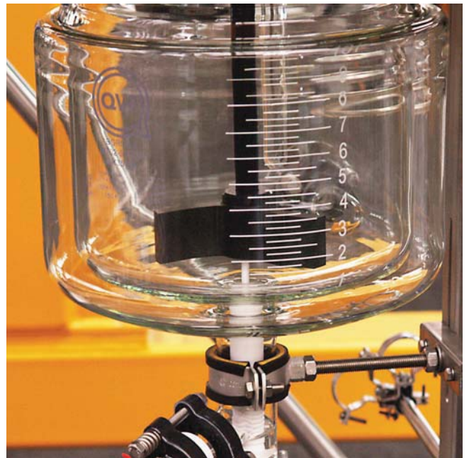
Illustr. 2: Bottom outlet valves with thermometer employed in a jacketed vessel
