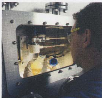
▲ De Dietrich glove box for sampling
