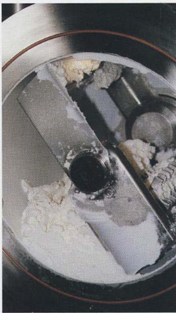
▲ Rosenmund agitator equipped with high speed dynamic choppers
