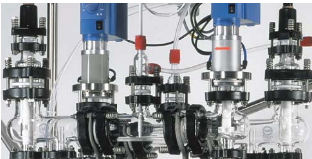
Fig.1: Settler with height-adjustable overflow (left), mixer head (right)
