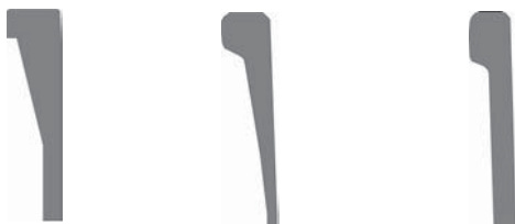
flat buttress end with groove, fire-polished (DN 15-DN 150)
